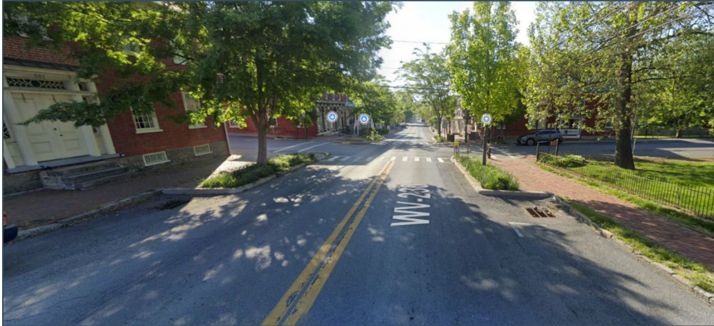
Existing vegetated curb extension in Shepherdstown Image Source: Google Maps, 2023
