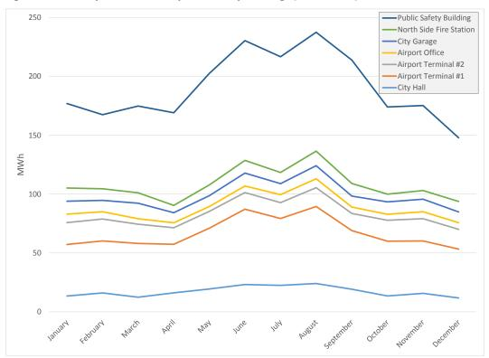
Figure 25: Monthly billed electricity use for City buildings (MWh, 2012)
