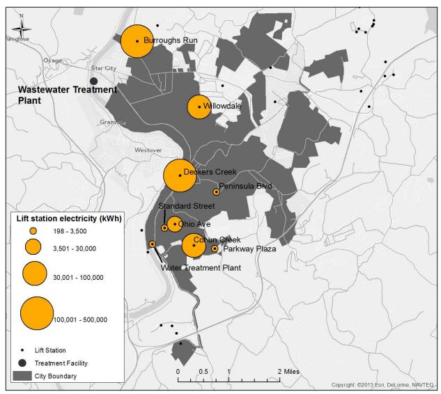
Figure 16: Electricity used by wastewater lift stations within the city of Morgantown
