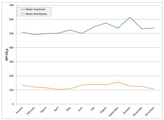
Figure 13: Total drinking water treatment and distribution emissions per month (MT CO<sub>2</sub>e, 2012)
